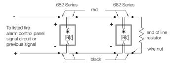
Polarity of signal circuit shown in supervisory state. On alarm the polarity reverses.
